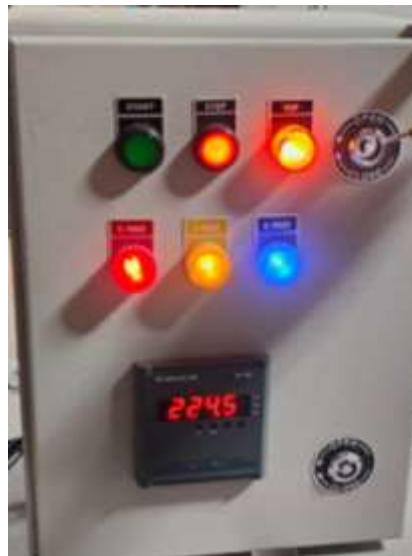
Fig 12: Trip Function of DOL Starter
